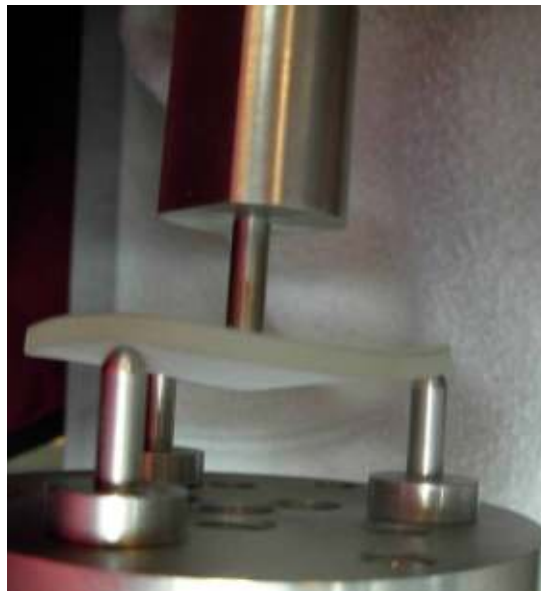
Fig. 5.8. Deflection of round plate with diameter of 29 mm under point load
