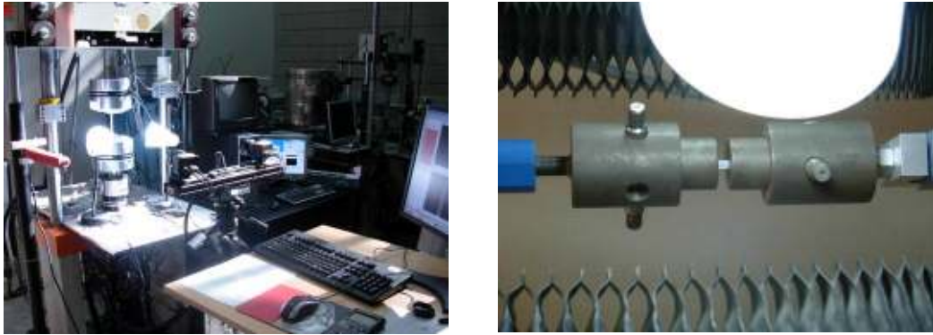
Fig. 2.3 Equipment set-up in tension and compression tests
