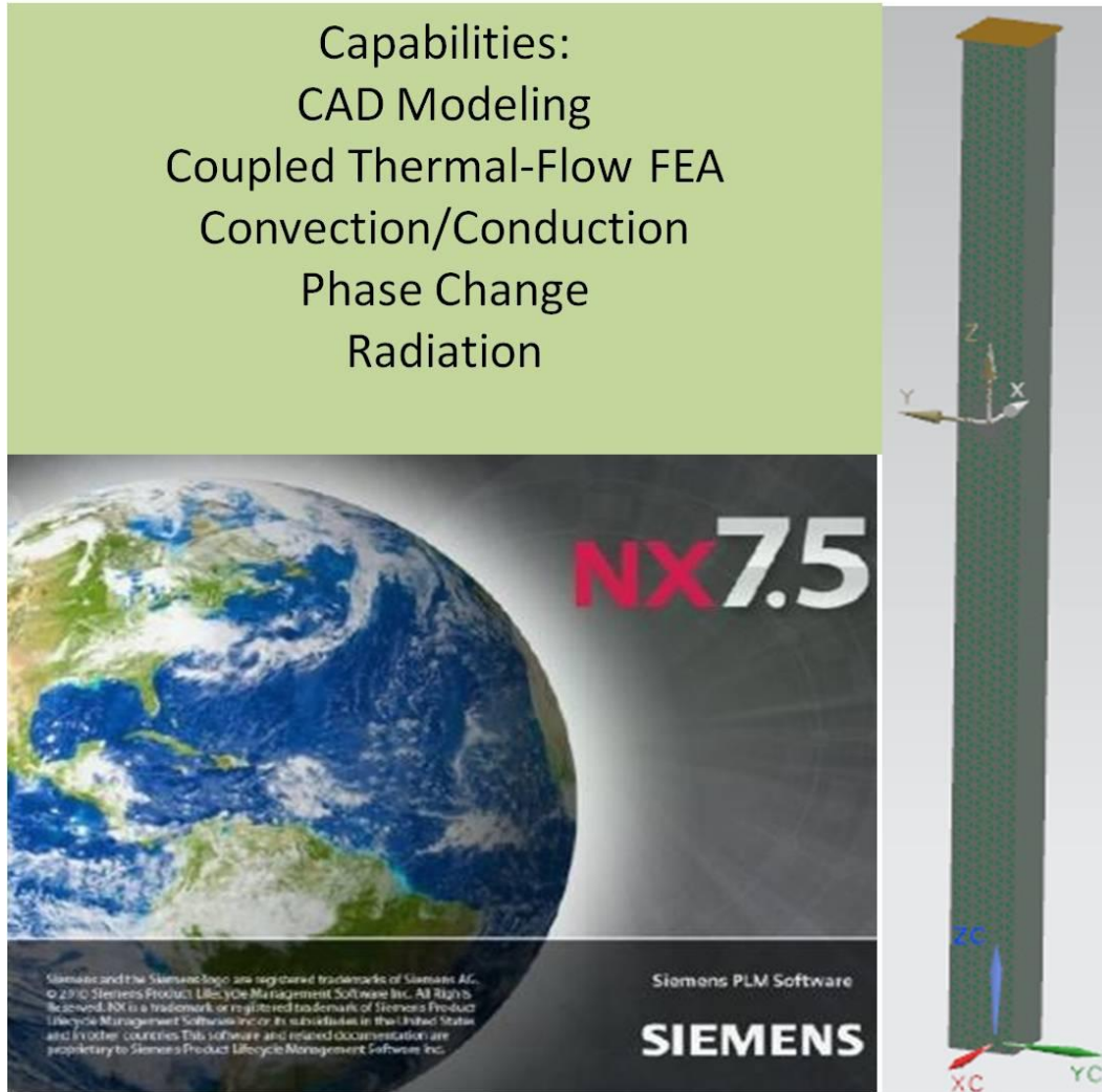
Figure 19. Relevant Siemens 7.5 CAD/FEA capabilities (left) and a sample image of a 2mm x 2mm x 35 mm open-top cuvette used in this analysis (right)
