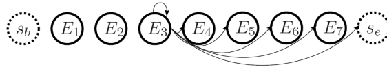
Fig. 4.1. (Extracted from [2]) Transitions for a traditional HMM model with 7 emitting states. Only transitions out of one state ( E_3 ) are displayed for clarity. In general, any state can have a non-zero probability specified for transitions to itself or to any state depicted to its right.
