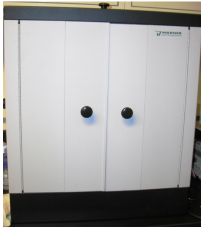
Figure 3.11: Faraday cage used to shield the nanopore chip and the electrodes from electrical noise.
