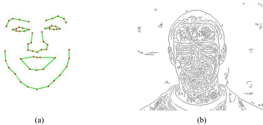
Figure 17: Results without semantic-aware processing: (a) Using only the matched face shape of Figure 16-(a); (b) Using the edge map of Figure 16-(a) generated from Canny edge detector with default parameters.
