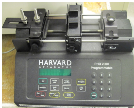
Figure 14. Harvard PHD 2000 programmable syringe pump
