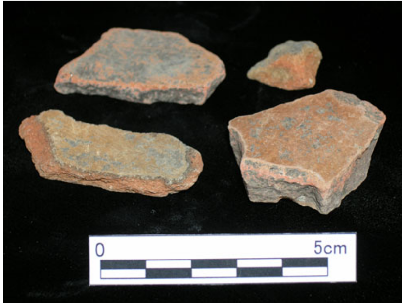
Figure 5.18. Examples of defective (misfired) sherds.
