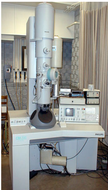
Fig. 2.8 Philips CM200 FEG TEM used at ASU (courtesy CSSS)
