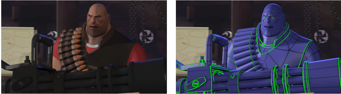
Figure 1.1: [Approximate Catmull-Clark patches rendered in Valve Software’s game: Team Fortress 2 ] The black lines indicate patch boundaries and the green lines provide crease support
