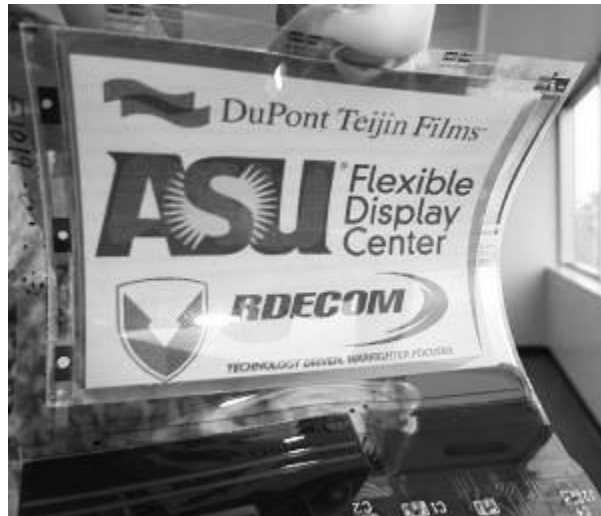
Figure 3.9 Example of an electrophoretic display that is built on flexible substrate HS-PEN using the temporary bond-debond process. The TFT array fabrication for the backplane utilized a bonded system consisting of HS-PEN, UV-PSA and the specialty carrier.
