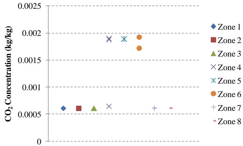
Figure A1.10: Tracer Gas Release in South AHU (5 min)
