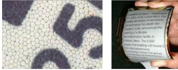
(a) Detail of colloidal suspension capsules (b) electrophoretic display on plastic
