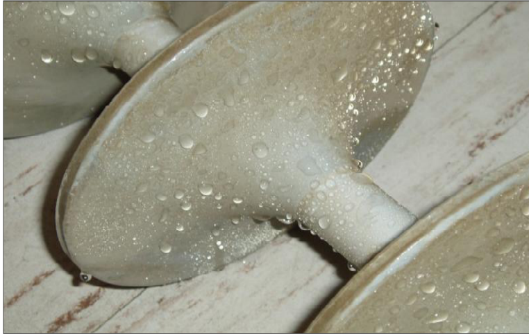
Figure 3. Composite insulator showing water droplets
