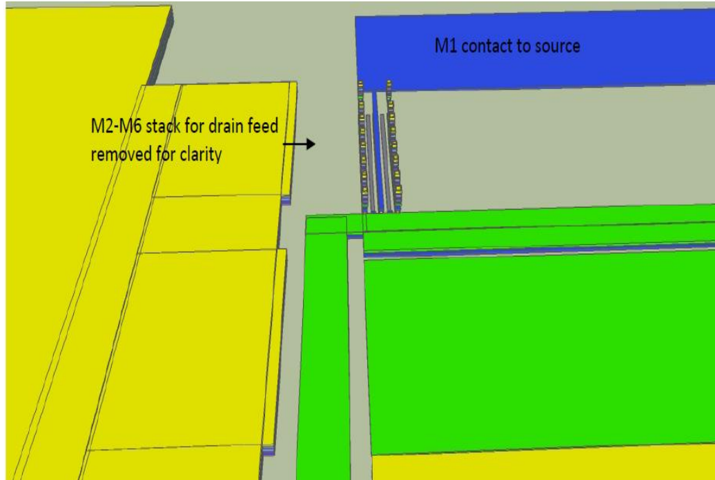
Fig. 103. Removes the entire drain line and some of the metal layers of the source and gate lines in Fig. 102 to show how individual fingers connect to the bus lines. All but two of the fingers were removed to simplify the picture.
