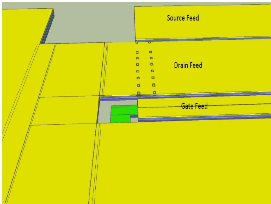
Fig. 102. Zooms in on one section of Fig. 101 to show the source, drain, and gate lines.
