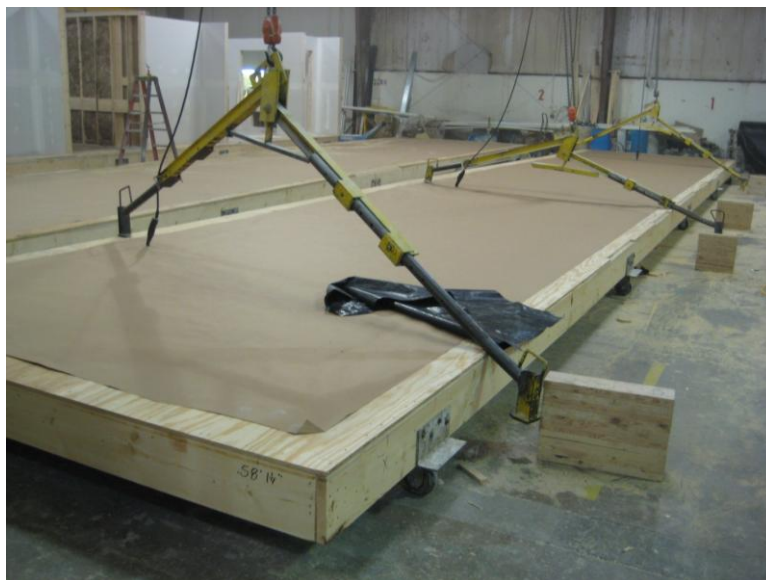
Figure 9. Completed floors being moved from jig to rollers.
