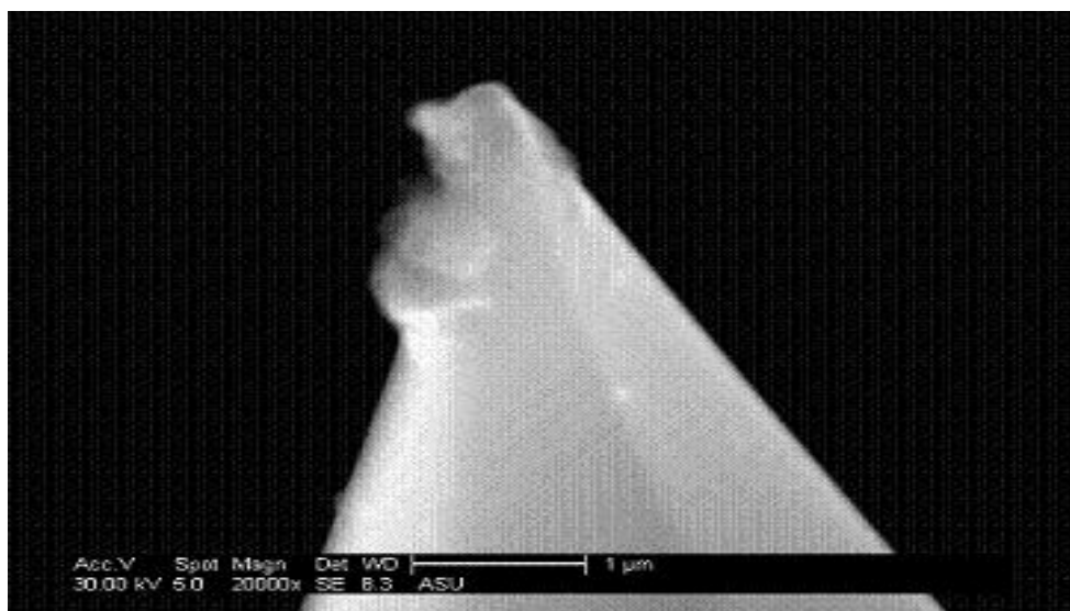
Figure 3.3. SEM image of AFM tip radius after metallic coating.
