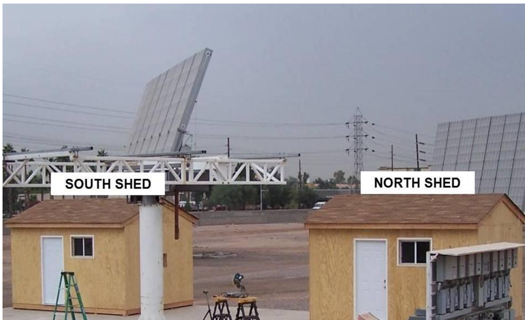
Figure 2.2 Experimental Setup of South (non BioPCM) Shed and North (BioPCM) shed
