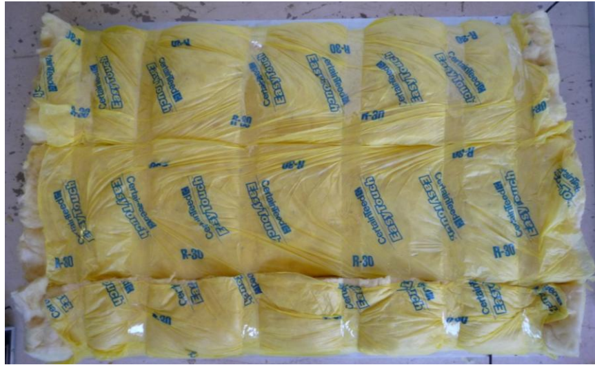
Figure 3.9 After covering the BAPV reference module with insulation material
