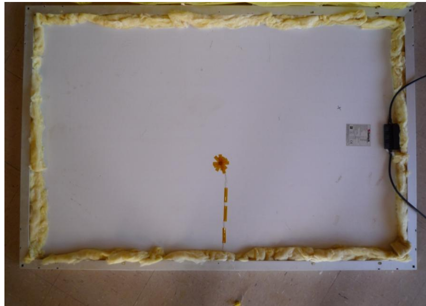
Figure 3.8 Before covering the BAPV reference module with insulation material
