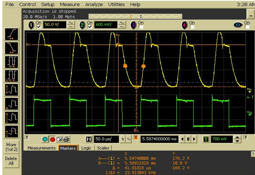
Fig. 20: Voltage Waveform for the JFET drain (yellow, 50V/div) and MESFET gate (green, 600mV/div) for a load current of 1.75 A_{RMS} and a temperature of 235°C.
