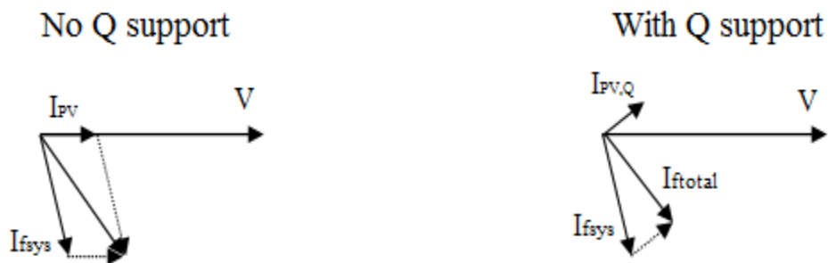
Fig. 5.16. Phasor diagram indicating decrease in fault current due to reactive power injection.
