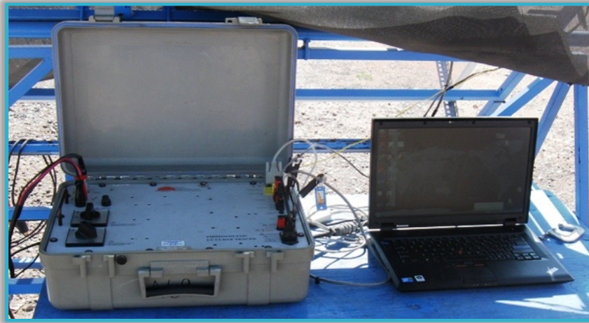
Figure 10. I-V Curve tracer Daystar DS-100C connected to laptop.
