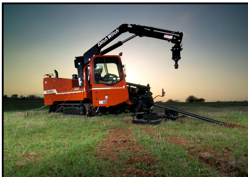
Figure 1.2 Medium Rig (Ditchwitch 8020)
