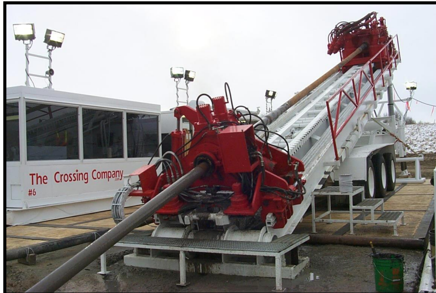
Figure 1.4 Heavy Large Rig (AA660)
