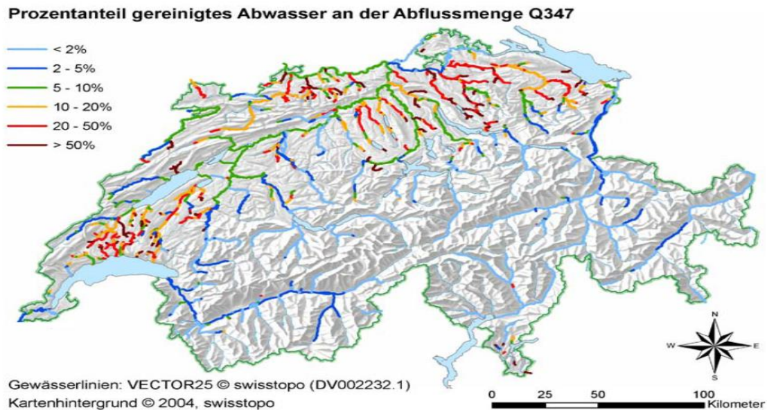
Figure 2.2 Geographical Distribution of Treated Wastewater in Streams under Dry Weather Low Condition (Q347) in Switzerland
