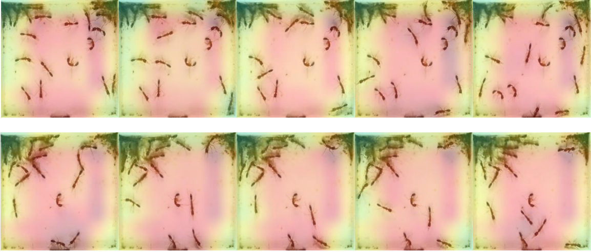
Figure 4.11: Two examples in two rows in each of which Grad-CAM heatmap is resized and superimposed on original RGB video frames sequentially sampled every second. Red regions have higher values while the blue lower values.
