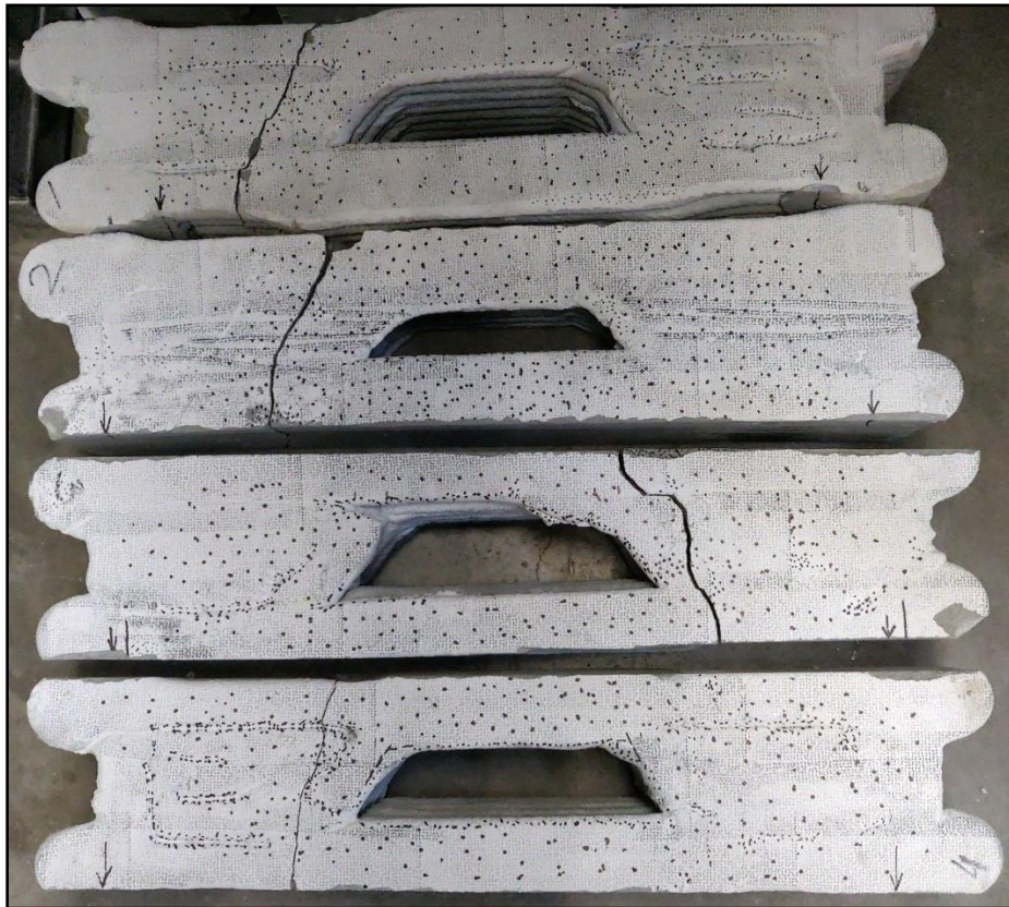
Figure 25. Failure modes of printed and casted beams in 2 nd generation.
