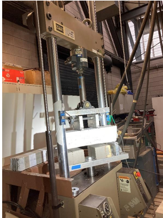
Figure 29. Apparatus utilized to test fiber beams under four-point bending.
