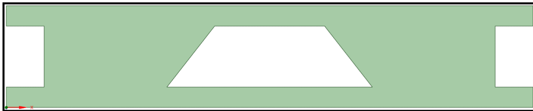
Figure 5. Results of removing small holes and smoothing edges for printability.
