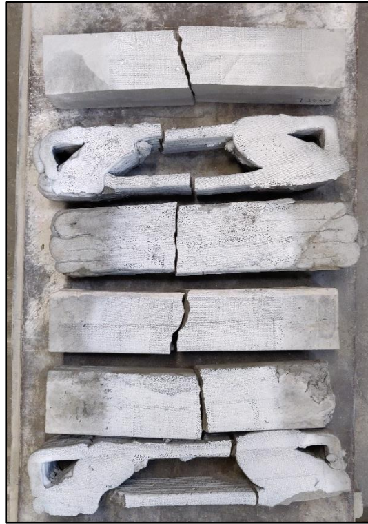
Figure 17. Failure modes of printed and casted beams in 1 st generation.
