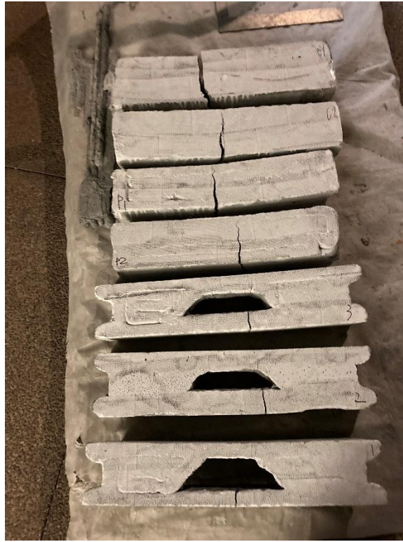
Figure 30. Failure modes of printed and casted fiber beams in 2 nd generation.
