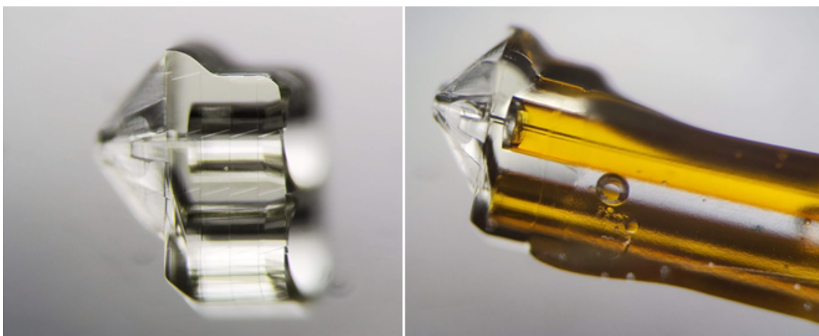
Figure A.18: (left): standalone nozzle, figure 3b (right): capillaries inserted into the nozzle. Top: liquid line, bottom: gas line.
