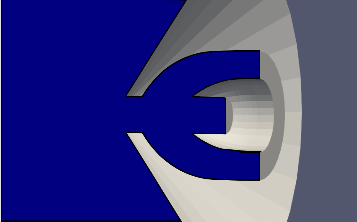
Figure 4.13: Computational flow field for the GDVN with bell-shaped geometry for gas flow field. Blue surface is the surface of symmetry.
