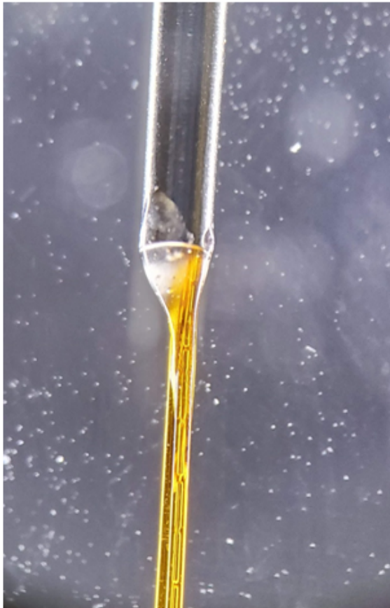
Figure A.20: (top): metal sleeve glued to nozzle/capillary, figure 5b (bottom): a visual on the approximate amount of glue needed at each end of the sleeve.
