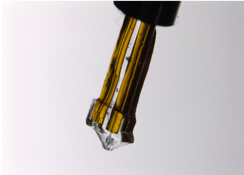
Figure 3.4: An assembled 3D printed nozzle.
