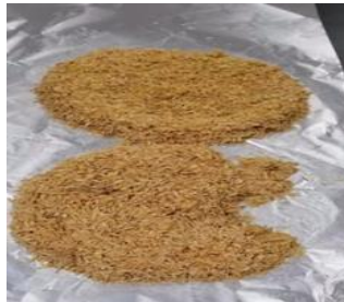
Fig 3.1: Acid washed rice husks
