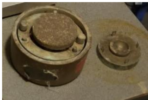
Fig 4.26: Ring with soil and porous stone
