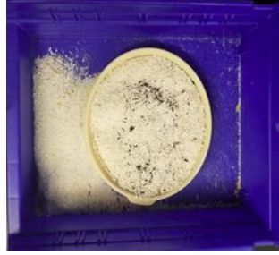
Fig 2.14: Rice husk ash/silica ash
