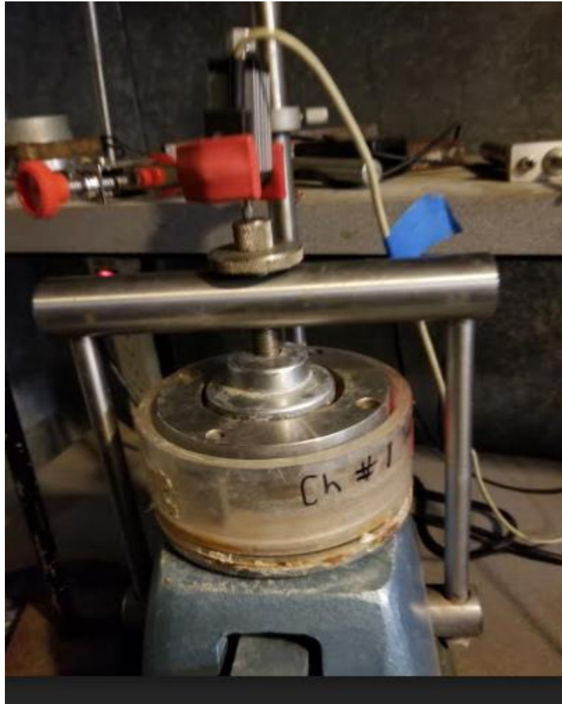
Fig 4.27: Odometer apparatus with LVDT and ring.
