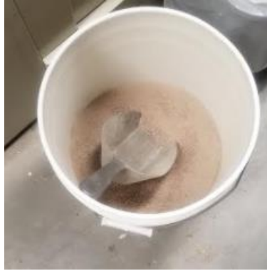
Fig 4.10: Anthem-bentonite clay after mixing
