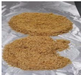
Fig 2.13: Acid washed rice husks
