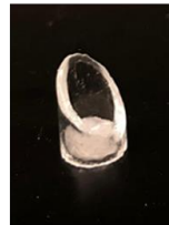
Figure 4.1. Device fabrication process and output results. Schematic of the 3D-printed molds, individual mold and mold array, (left top) and valve fabrication output (left bottom). The valve is composed of a hydrogel and surrounded by the glass needle to support the valve structure. 3D-printed molds are assembled in the needle then the liquid hydrogel solution is cured by UV light for 4 mins at 365 nm wavelength to be solidified. The solidified molds are detached from the hydrogel and submerge the device into the water to prepare for the functionality test (Right).
