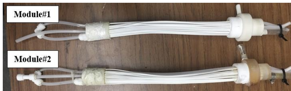
Figure 10. A Schematic Diagram (Top), and a Photograph (Bottom) of the ETC–MD Modules.
