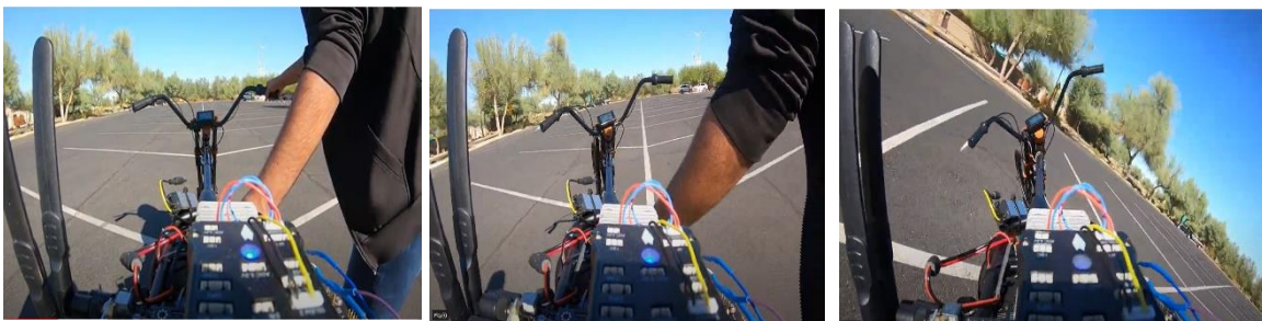
(a) Initial start condition (b) Self-balancing condition (with rolling) (c) Bicycle failing condition
