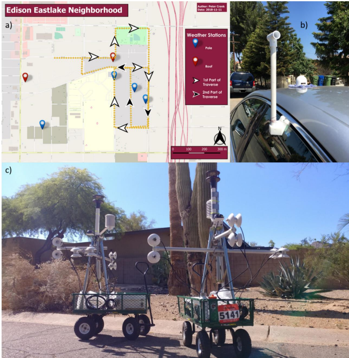
Figure 8 – Map of the route traverse with traverse instruments. A) shows the route for the traverses, b) is the car traverse thermocouple, and c) shows the two MaRTy carts, as developed by Ariane Middel. The traverses in this neighborhood only used one of the two carts.
