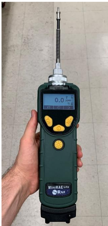
Figure 2.4 A commercially available handheld MiniRae Lite PID monitor by RAE Systems Inc.
