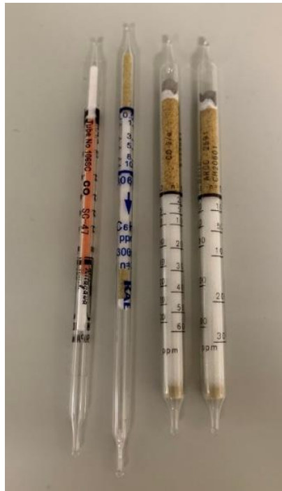
Figure 2.11 Portable colorimetric tubes by RAE Systems Inc. and Draeger for detection on carbon monoxide and benzene.
