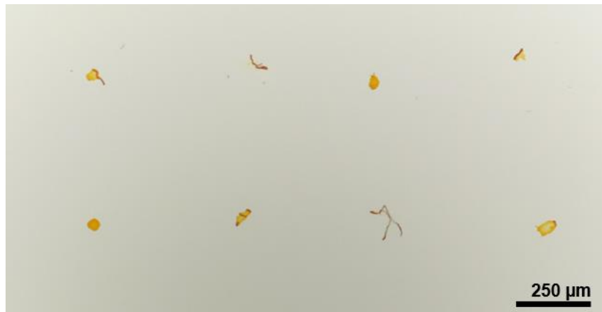
Figure 5.5 Sensors that are cracking, peeling, and delaminating from the surface of a CMOS imager treated with TCS (same printing formulation as Figure 5.4).
