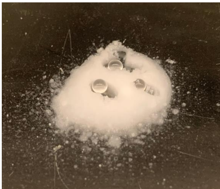
Figure 5.1 Enova hydrophobic aerogel IC3100 fine particles from Cabot Aerogel with water droplets resting on top illustrating its hydrophobicity.
