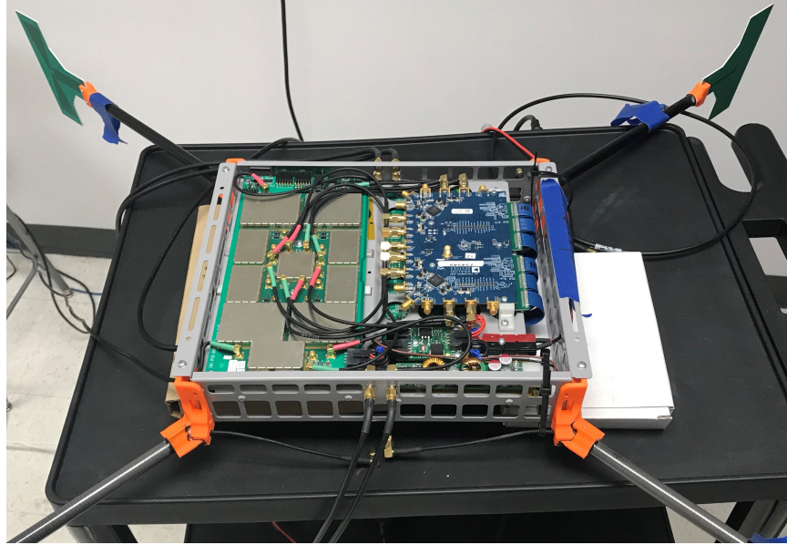
Figure 7.1: COTS Experimental Hardware Mounted In An Aluminum Frame. The Amplifier And Transmit-Receive Switching Board (Left) Is Shielded With Modular Copper Plating. The RF Board (Blue, Right) Sits On Top Of The Motherboard Underneath. The Antennas (Top Left And Right) Are Mounted To Carbon Fiber Tubes Through Which RF Feeds Are Fed And Connected To The Amplifier Board.
