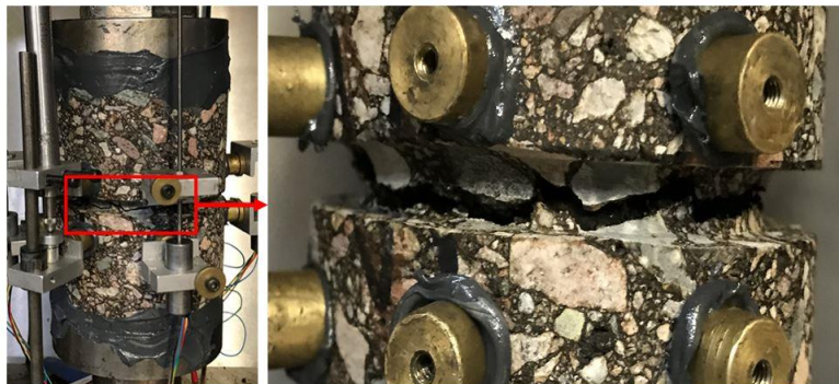
Figure 5-5. Photo of Sample Failure and Crack Plane Under Direct Tension Test.
