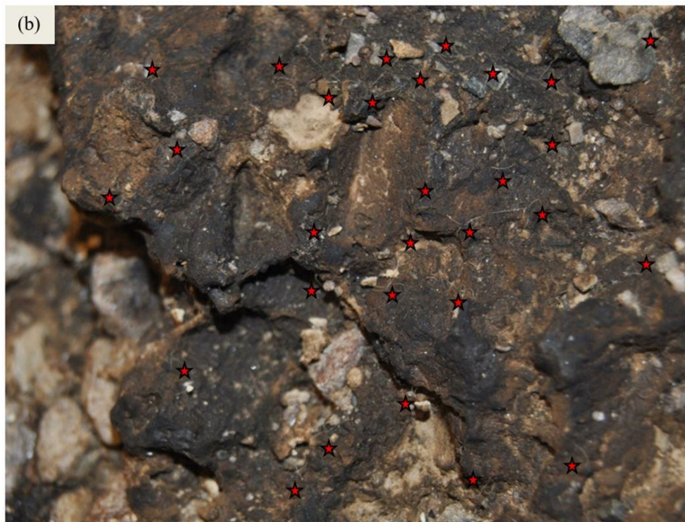
Figure 3-12. Photos Taken from the Aramid Fibers Distributed on the Surface Fracture of Each FB Mix; (a) Overall View of Casting Surface and (b) Enlarged Photo of Central Section.
