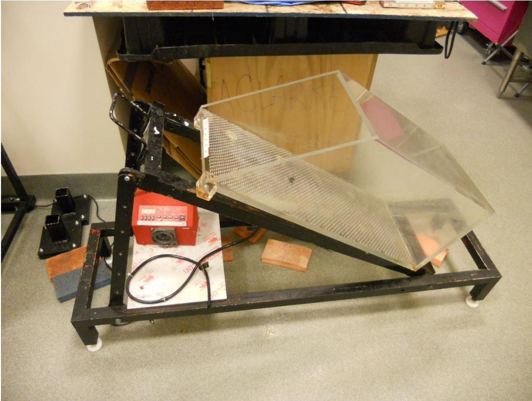
Figure 5: Experiments were conducted in a 76 x 30 cm plexiglass tank with a fitted 4mm grid steel mesh. The tank sat on an adjustable apparatus capable of producing the \sim 7 , 16, and 29^\circ slopes necessary. The distance from the vent to the back of the tank was 50 cm.
