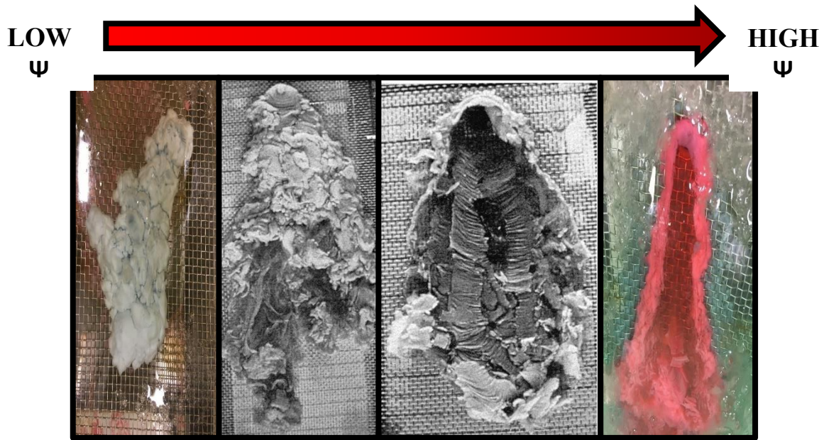
Figure 4: Four primary morphologies observed by Fink and Griffiths [1990] and their relation to \Psi . A fifth morphology (No Crust, not pictured here) was observed beyond Levees and may be appropriate to some systems. Approximate \Psi value ranges of morphologies observed in our experiments are as follows: Pillows ( \leq 2 ); Rifts (4 – 12); Folds (15 – 29); Levees (34 – 54); No Crust ( >55 ). Values in-between frequently result in transition morphologies, defined here as morphologies that form contemporaneously. Blurriness in colorized lab images due to ice.
