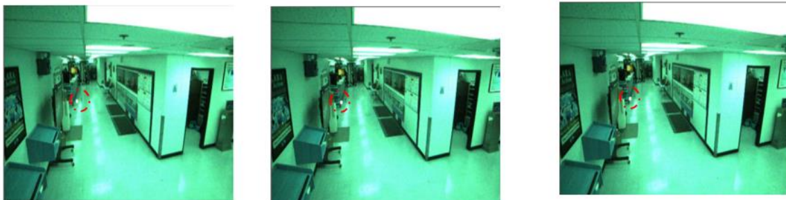
Figure 20 False Detection due to Reflective Objects (Red Circle the False Detection, the Algorithm Detected One Worker in the Video, whereas there is No Worker)
