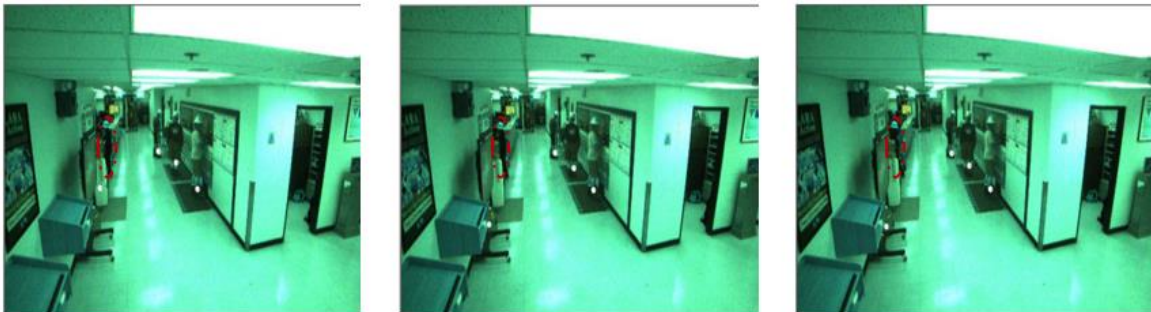
Figure 21 Occlusions due to the Background Obstacles. (The Algorithm Missed the Worker at the Left.)
