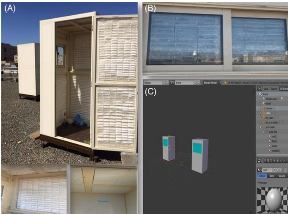
Figure 4.1: (a) Appearance of Experimental Field-test, (b) Window With PCM and (c) Simulation Model.
