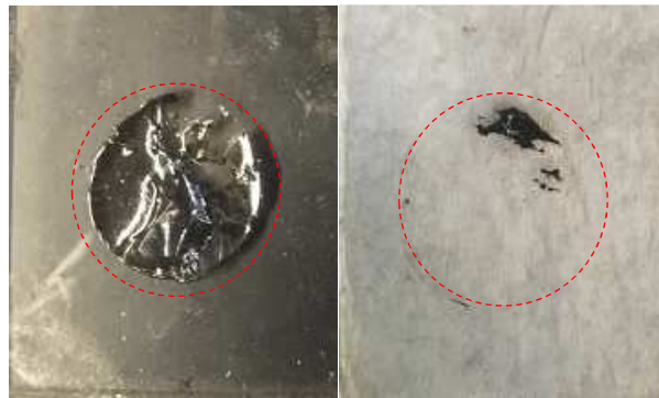
Figure 4-3 Binder Residue From Bitumen Sample R (Left) Adhering to the Glass Surface in Dry Condition; (Right) after Adhesive Failure Following 2 hr Water Conditioning
