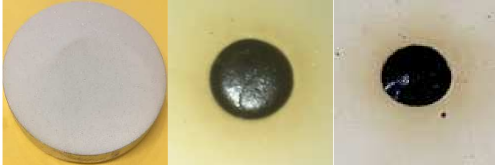
Figure 5-2 (Left) Glass Beads Used to Mix with Bitumen; (Middle) Sample Before Water Conditioning; (Right) Sample after Water Conditioning
