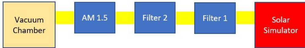
Figure 3.8: Schematic for the arrangement of NDF's and AM 1.5 filter
