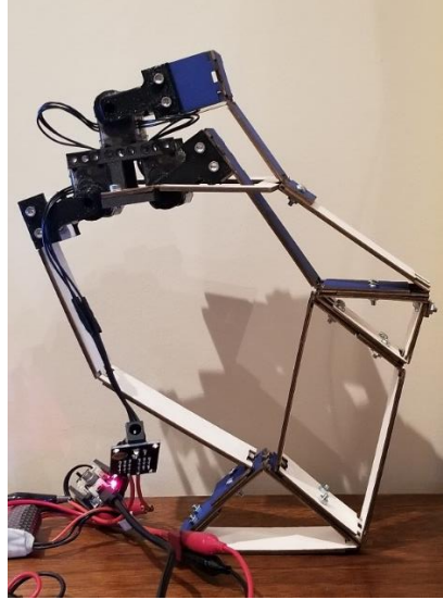
Figure 2: Biped leg design for the robot platform [5].
