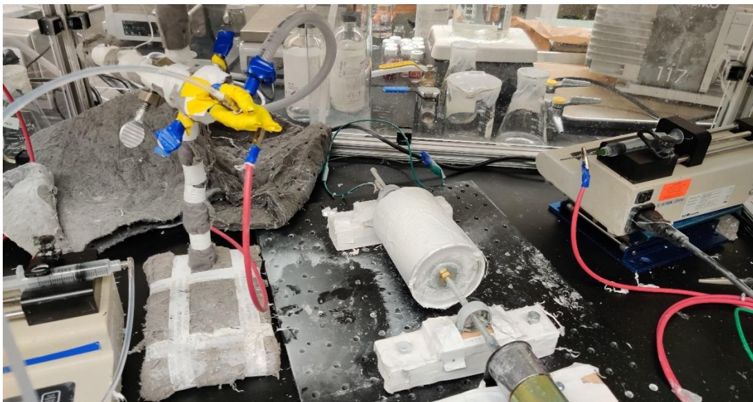
Figure 15. Modified dual electrospinning setup.
