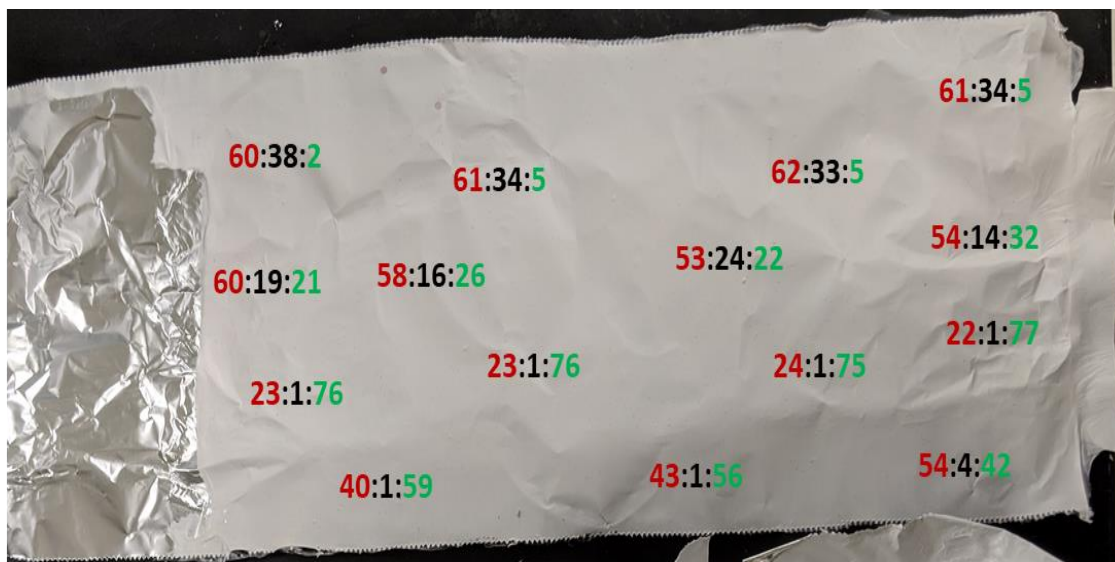
Figure 6: Elemental map collected from 15 locations in a co-spun mat containing PVA and PVC, where carbon (-C) is represented by red , oxygen (-O) by black and chlorine (-Cl) by green . The data mapped gives the weight percent composition in the format (C:O:Cl) .
