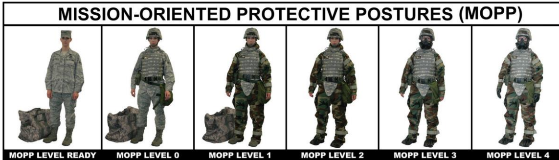
Figure 1.1 Illustration of the MOPP levels highlighting the required additional garments warfighters need to carry and wear to protect against potentially hazardous conditions. 22
