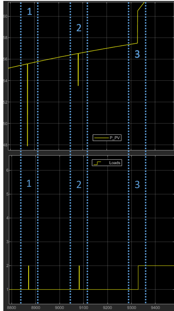
Figure 4.4. Example of MPPT Operation for Feedback-based Control.
