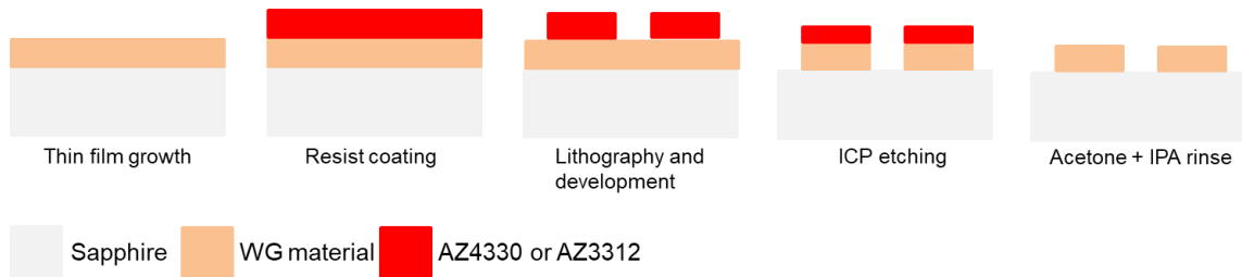
Figure 3-1. The fabrication process of GaN waveguide in the initial stage of this research.
