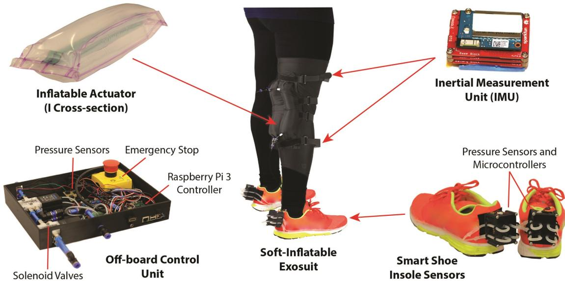
**Figure 3.1** (a) Inflatable Actuators of I Cross-section. (b) Off-board Control Unit. (c) Imus on the Exosuit (d) *Smart Shoe* Insole Sensors.
