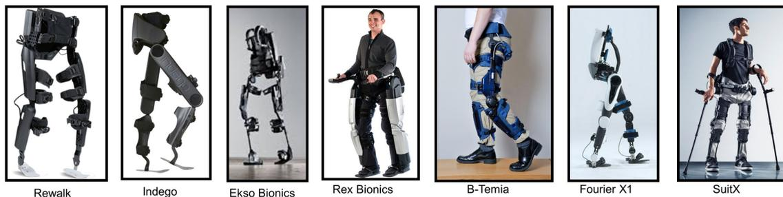
**Figure 1.1** Commercially Available Exoskeletons for Gait Rehabilitation.
