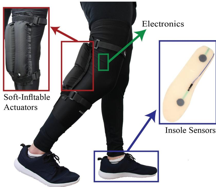
**Figure 2.6** Design of the Soft-inflatable Exosuit. Inflatable Actuators Are Encased in a Fabric Sleeve with the On-board Electronics in a Separate Pouch. FSR Based Insole Sensor Are Placed in the Shoes.
