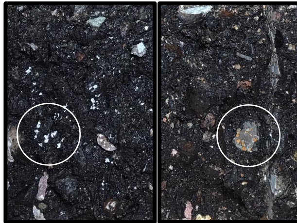
Figure 5- 2 a) Salt Water Conditioned Sample, b) Acidic Water Control Conditioned
