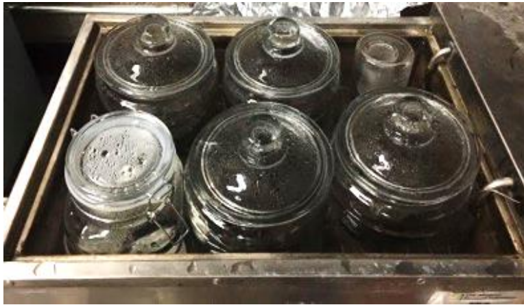
Figure 5- 1 Containers for Conditioning Samples in Salt and Acidic Water
