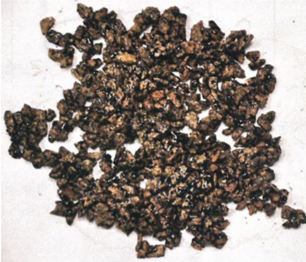
Figure 2- 7 Sample with Major Moisture Stripping after the Texas Boiling Test (Liu et al., 2014)
