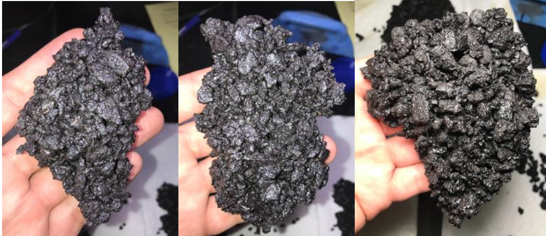
Figure 6- 8 Control, MMT-doped, and PET-doped (left to right) Samples after Boiling Water Test
