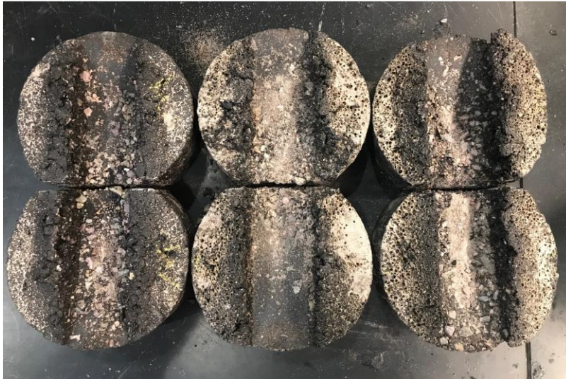
Figure 6- 12 MMTa-doped, MMTc-doped, and MMTb-doped Mixtures (left to right) after the Hamburg Wheel Tracking Test
