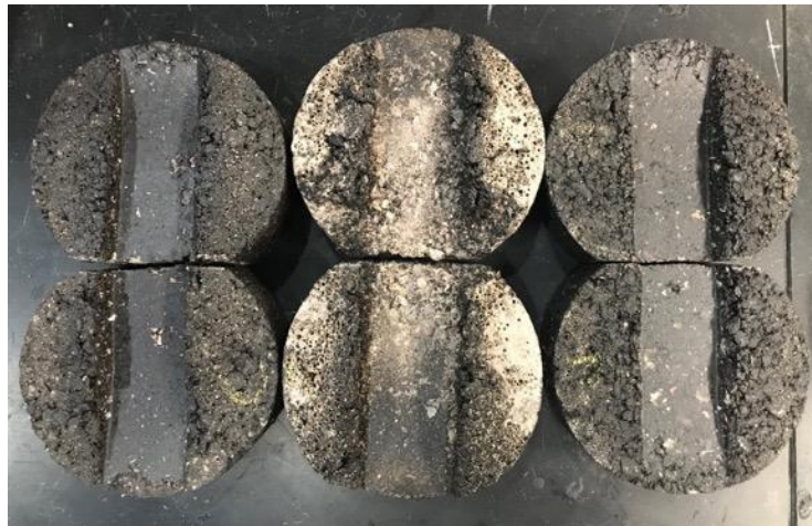
Figure 6- 11 Control, MMT c -doped, and PET-doped Mixtures (left to right) after the Hamburg Wheel Tracking Test
