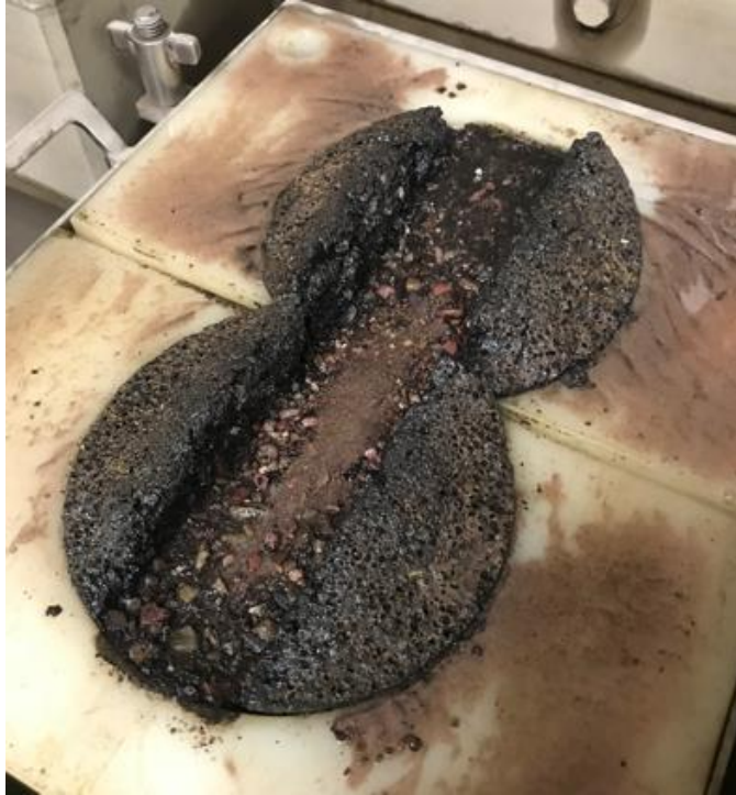
Figure 2- 2 Asphalt Mixture with Major Moisture Stripping
