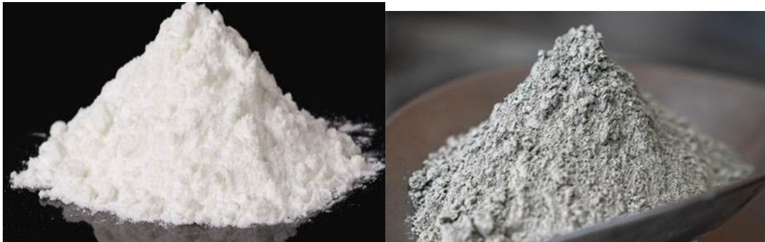
Figure 2- 9 Hydrated Lime (left) and Cement (right)
