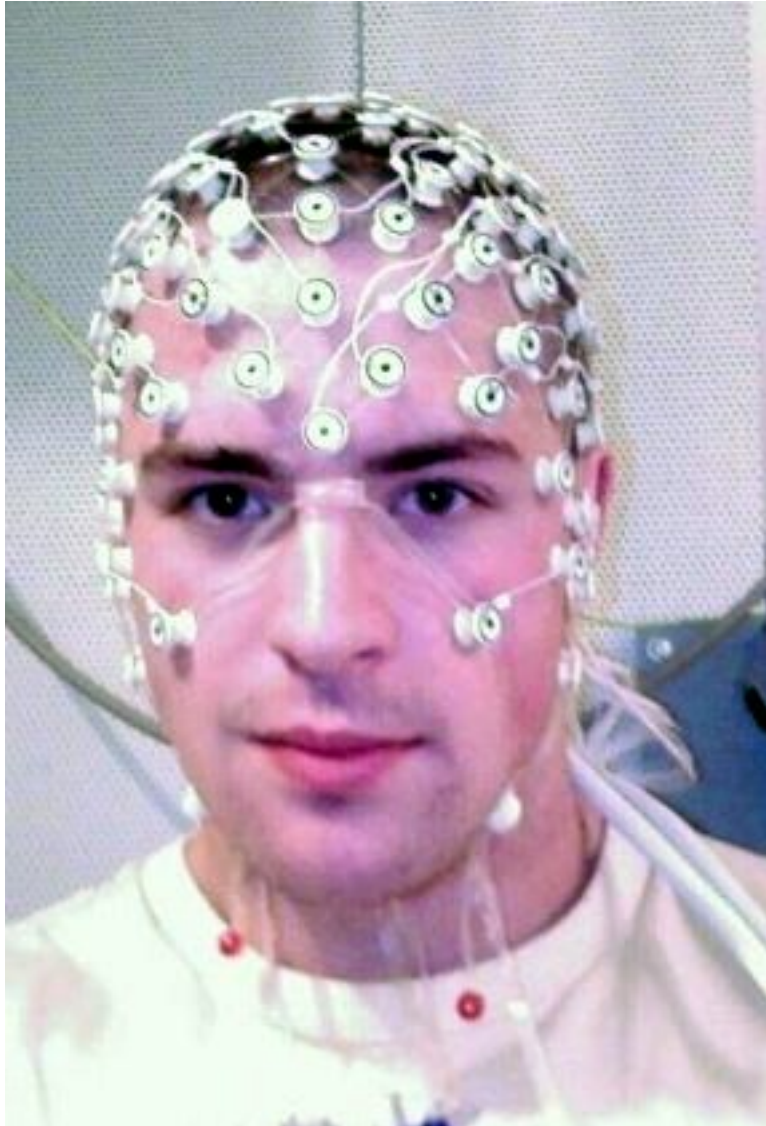
Figure 1.2: Subject with EEG electrodes ready for measurements; a far less intrusive alternative to brain investigations. Image by Douglas Myers, Public Domain.
