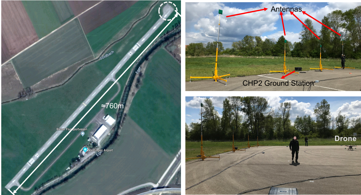
Figure 9.5: Depiction of flying test setup on the end of airport runway.
