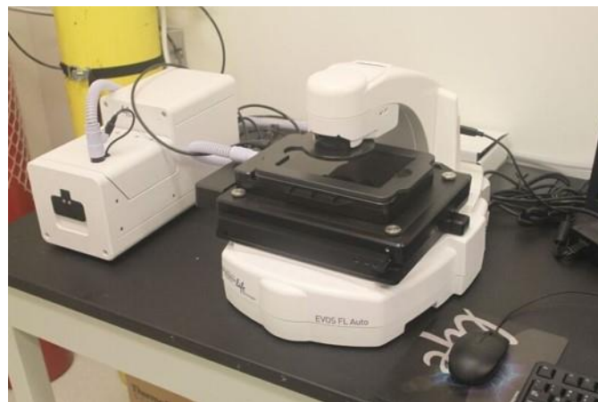
Figure 15 - Image of EVO live cell imaging microscope used to image ejection of fluorescein into aCSF infused agar
