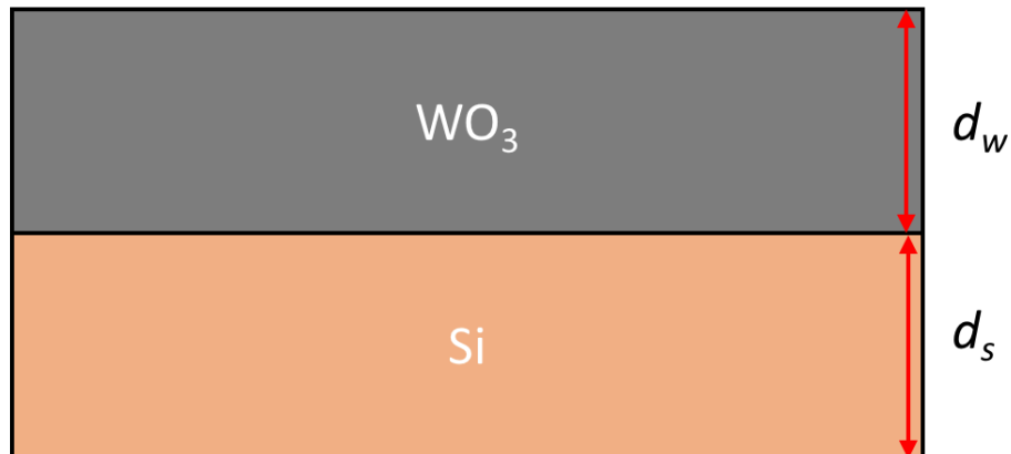
Figure 4.4: A layer of tungsten trioxide varies from 20 nm to 200 nm in steps of 20 nm on a 200 nm thick layer of silicon.
