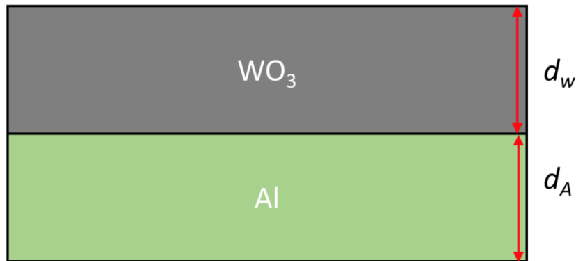
Figure 3.2: Simple schematic of tungsten trioxide, WO 3 which varies in thickness from 40 nm to 200 nm. This is deposited on a 200 nm thick aluminum, Al wafer. Aluminum at this thickness is opaque so that transmittance will be zero.
