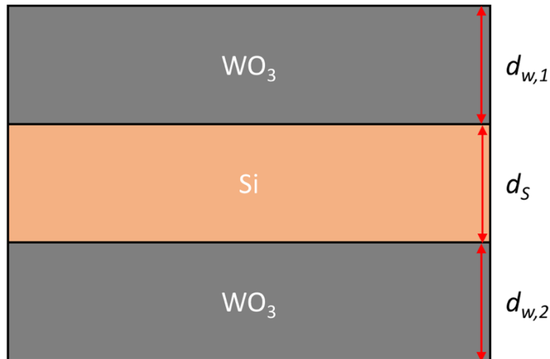
Figure 4.8: A top layer of tungsten trioxide, WO 3 varies from 20 nm to 200 nm, a middle layer 50 nm thick silicon, and a bottom layer of WO 3 vary from 20 nm to 200 nm.
