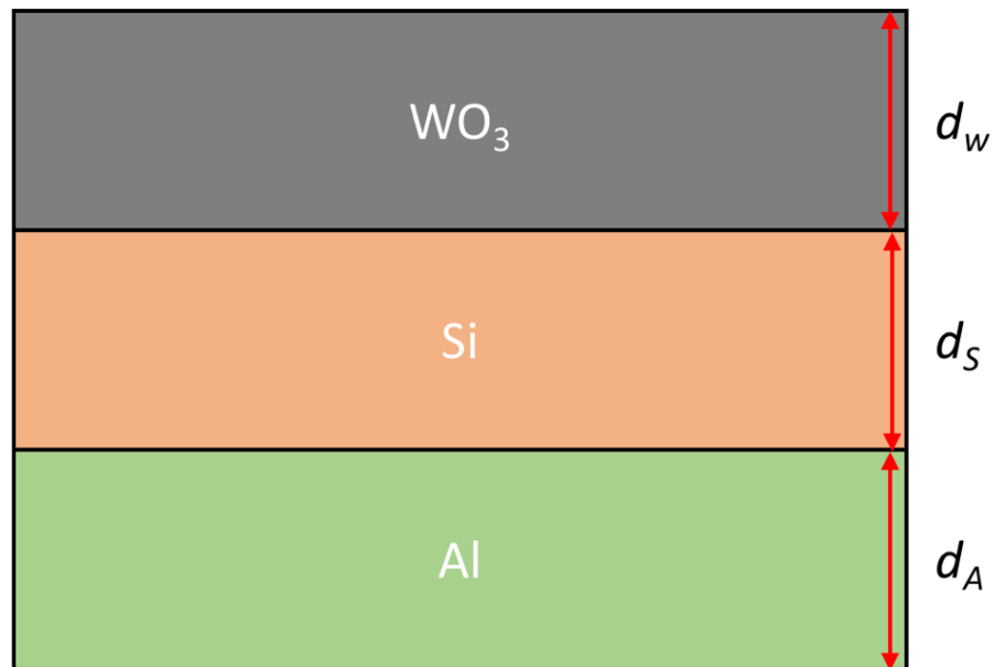
Figure 3.6: Simple schematic of tungsten trioxide WO_3 which varies in thickness from 20 nm to 200 nm, the second layer is 50 nm of silicon Si , and the base is 200 nm of aluminum Al wafer. Aluminum at this thickness is opaque so that transmittance will be zero.
