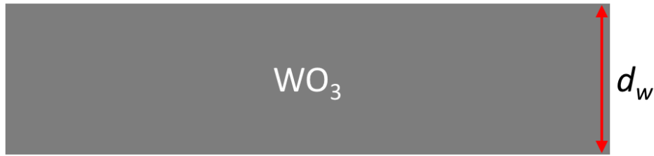
Figure 4.1: A single layer of tungsten trioxide varying from 20 nm to 200 nm, in steps of 40 nm.
